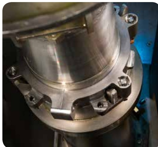
Flow control collar seals slip joint assembly and provides lateral support while allowing thermal growth
