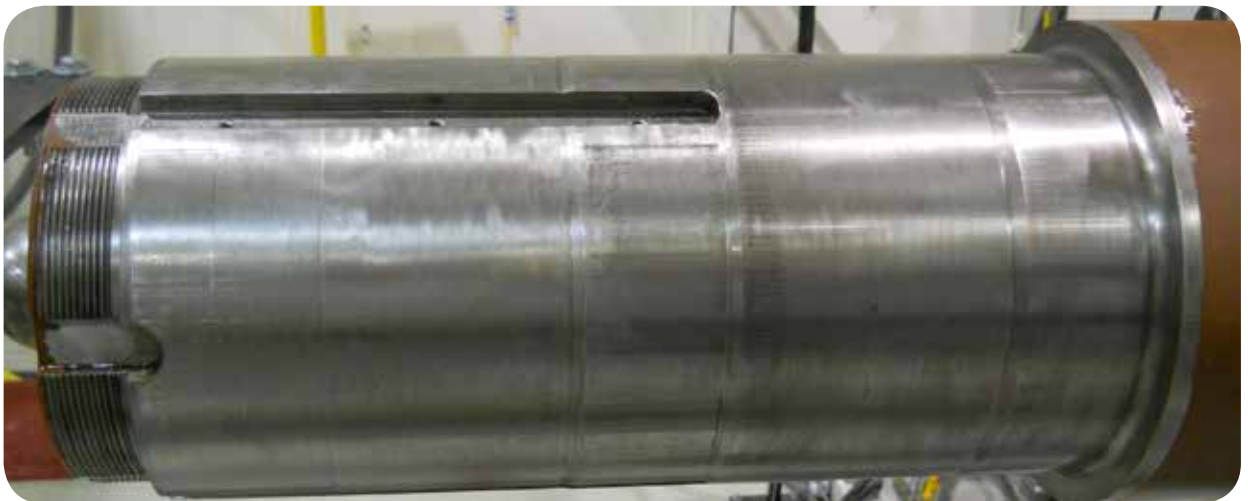
Flywheel fit area of motor shaft showing wear. This condition may be detected during operation with vibration monitoring.
