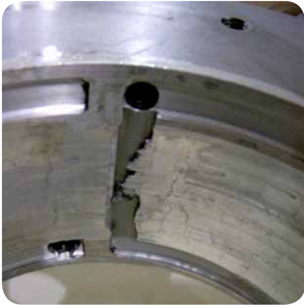
Reactor recirculation pump motor bearing damaged from oil whirl. Detectable before the failure and after, and preventable if identified promptly.
