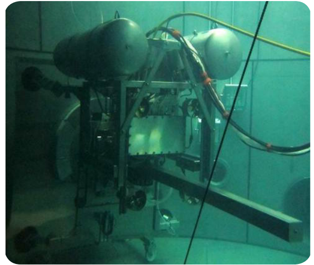
Floats above the manipulator add buoyancy so the props can swim from nozzle to nozzle without aid of the polar crane.
